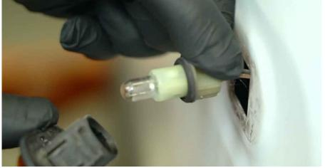
3 Attach the bulb holder to a new side indicator light.
