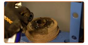
Press a new bearing into the wheel hub. Use a bush and bearing driver set.
