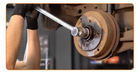
10 Remove the brake drum.
