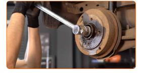
10 Remove the brake drum.
