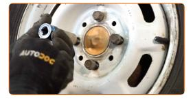
Lower the car and working in a cross order, tighten the wheel bolts. Use a torque wrench. Tighten it to 90 nm torque.
