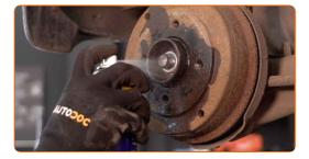
Unscrew the wheel hub axle nut. Use a drive socket #30. Use a tap wrench.
