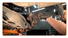
10 Remove the brake caliper.
