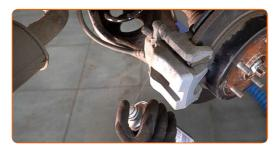
Unscrew the brake caliper fastening. Use a drive socket #14. Use a ratchet wrench.
