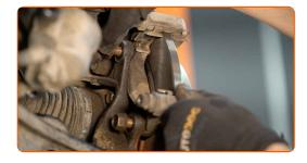
Tighten the brake caliper bracket. Use a drive socket #17. Use a torque wrench. Tighten it to 88 Nm torque.
