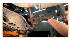
10 Remove the brake caliper.
