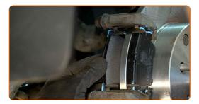
Install the brake caliper and fix it. Use a drive socket #14. Use a torque wrench. Tighten it to 27 Nm torque.
