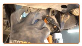
Unscrew the fastener connecting the control arm to the rear knuckle. Use a combination spanner #17.
