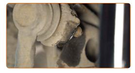
17 Remove the arm. Use a ball joint puller.
