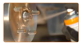
Clean the brake disk surface. Use all-purpose cleaning spray.
