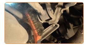
Unscrew the arm fastening to the beam. Use a combination spanner #17 (2 pieces).
