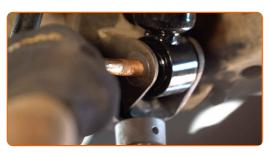
Tighten the lower fastener of the shock absorber. Use a combination spanner #17. Use a torque wrench. Tighten it to 80 nm torque. Use a crowbar.
