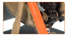
Unscrew the lower fastener of the shock absorber. Use a drive socket #17. Use a combination spanner #17.
