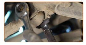
Remove the fastening bolt. Use a crowbar.
