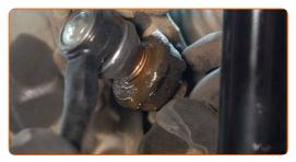
Tighten the fastener connecting the suspension arm to the rear knuckle. Use a combination spanner #17. Use a torque wrench. Tighten it to 90 nm torque.
