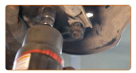
Tighten the ball joint fastener. Use a drive socket #17. Use a torque wrench. Tighten it to 92 nm torque.
