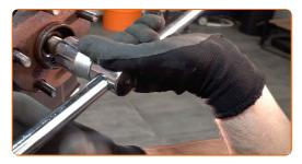
Treat the splines of the driveshaft CV joint. Use WD-40 spray.
