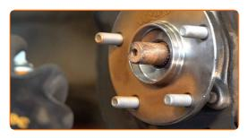
36 Install the brake disc.
