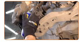
Unscrew the caliper bracket fastening. Use a drive socket #17. Use a tap wrench.
