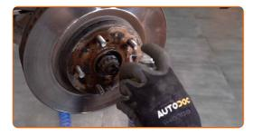
14 Remove the brake disc.
