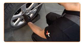
Restake the fastener of the driveshaft. Use a flat metal-working chisel. Use a hammer.
