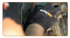
Tighten the brake caliper bracket. Use a drive socket #18. Use a torque wrench. Tighten it to 98 nm torque.
