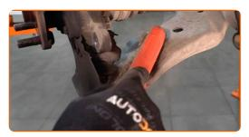
Unscrew the fastener connecting the ball joint to the suspension control arm. Use a drive socket #17.
