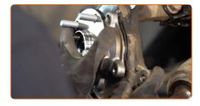
Tighten the wheel hub bearing fasteners. Use a drive socket #17. Use a ratchet wrench.
