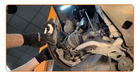
Remove the brake disc.
