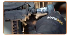
10 Remove the brake caliper.
