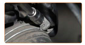
Screw in the fasteners of the air filter housing. Use a drive socket #10. Use a ratchet wrench.
