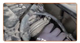
Screw the fastening clamp connecting the air duct to the air filter housing. Use a drive socket #10. Use a ratchet wrench.
