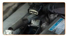
Unscrew the fasteners of the ignition coils. Use a drive socket #10. Use a ratchet wrench.
