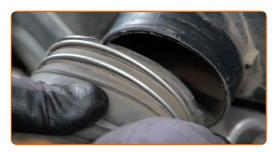
Unscrew the fasteners of the air filter housing. Use a drive socket #10. Use a ratchet wrench.
