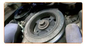
Pull aside the V-ribbed belt tensioner pulley. Use a drive socket #19.
