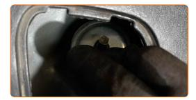
Screw the upper fastener of the shock absorber.
