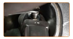
Treat the upper fastener of the shock absorber. Use copper grease.
