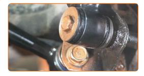
Install the elements of the shock absorber upper mount.
