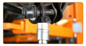
Unscrew the upper fastener of the shock absorber.
