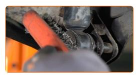
Unscrew the lower fastener of the shock absorber. Use a drive socket #14. Use a ratchet wrench.
