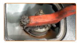
Loosen the upper fastener of the shock absorber. Use a combination spanner #14 (2 pieces).
