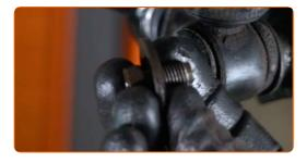
Support the rear knuckle. Use a hydraulic transmission jack.
