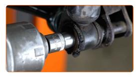
Remove the fastening bolt.
