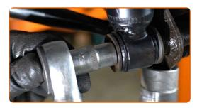
Treat the lower fastener of the shock absorber. Use copper grease.
