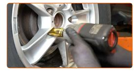
Lower the car and working in a cross order, tighten the wheel bolts. Use wheel impact socket #19. Use a torque wrench. Tighten it to 103 Nm torque.
