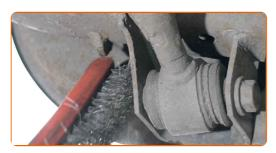
Clean the fastener connecting the sway bar link to the suspension arm. Use a wire brush. Use WD-40 spray.
