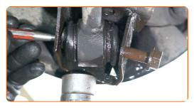
Make a mark on the camber adjustment bolt.
