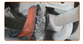
Unscrew the fastener connecting the stabilizer link to the control arm. Use a drive socket #17. Use a ratchet wrench.
