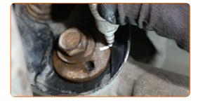
Unscrew the fastener connecting the control arm to the subframe. Use a combination spanner #17. Use a drive socket #17. Use a ratchet wrench.
