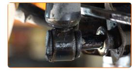
Unscrew the fasteners of the bracket that connects the shock absorber to the rear knuckle. Use a drive socket #14. Use a ratchet wrench.
