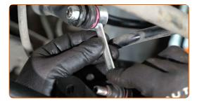
Screw in the fastener that connects the sway bar link to the suspension arm.
