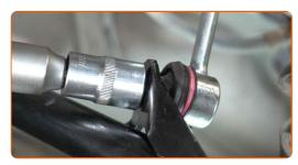
Clean the mounting seat of the bracket. Use a wire brush. Use WD-40 spray.
