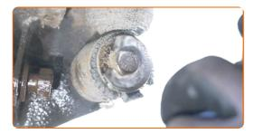
Clean the fasteners of the bracket that connects the shock absorber to the rear knuckle. Use a wire brush. Use WD-40 spray.
