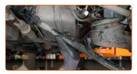
Clean the suspension arm mounting seats. Use a wire brush. Use WD-40 spray.
