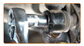
Remove the fastening bolt.
