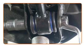
Tighten the fastener connecting the control arm to the subframe. Use a combination spanner #17. Use a drive socket #17. Use a torque wrench. Tighten it to 113 Nm torque.
