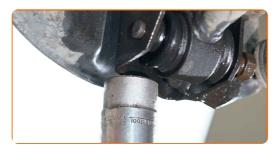
Clean the lower shock absorber fastener. Use a wire brush. Use WD-40 spray.
