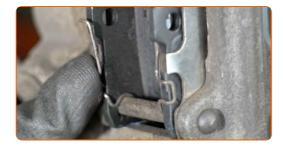
26 Install the brake pad retaining clip.
