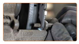
Install the retaining springs of the brake pads. Use a flat screwdriver.
