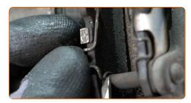
Clean the brake pad guide pins. Use a wire brush. Use a brake cleaner.
