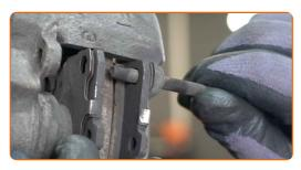
11 Remove the brake pads.
