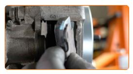
Install the brake pad guide pins.
