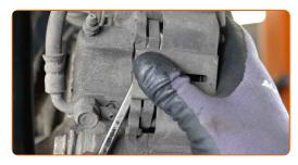
Remove the retaining springs of the brake pads. Use a flat screwdriver.
