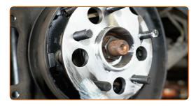
20 Install the brake disc.
