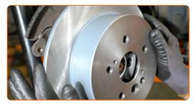
Set the parking brake adjuster in the correct position. Use a flat screwdriver.
