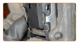
Install the brake caliper retaining spring.
