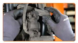
Tighten the brake caliper fasteners. Use a drive socket #14. Use a torque wrench. Tighten it to 44 Nm torque.
