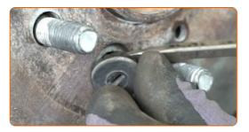
Release the parking brake adjuster. Use a flat screwdriver.
