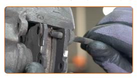
11 Remove the brake pads.
