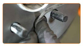
Treat the brake caliper pistons. Use a nylon cleaning brush. Use a brake cleaner.
