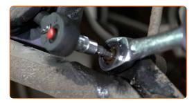
Unscrew the fastener connecting the stabilizer link to the stabilizer bar. Use a combination spanner #14. Use HEX No.H5. Use a ratchet wrench.
