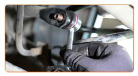
Screw in the sway bar link fasteners. Use a combination spanner #17. Use HEX No.H5. Use a ratchet wrench.
