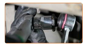
Tighten the fastener connecting the sway bar link to the suspension arm. Use a drive socket #17. Use a torque wrench. Tighten it to 44 Nm torque.
