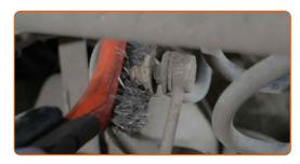
Unscrew the fastener connecting the stabilizer link to the control arm. Use a combination spanner #14. Use HEX No.H5. Use a ratchet wrench.
