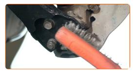
Unscrew the fasteners connecting the ball joint to the control arm. Use a drive socket #17. Use a ratchet wrench.
