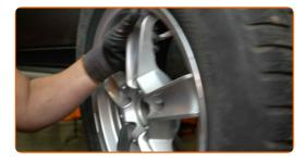
Unscrew the fastener connecting the drive shaft to the wheel hub. Use 12-point socket No.30. Use a ratchet wrench.
