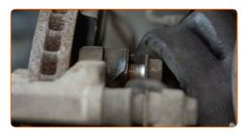
Screw in the fasteners of the brake caliper bracket. Use a drive socket #17. Use a ratchet wrench.
