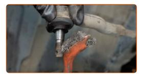
Clean the ball joint fasteners. Use a wire brush. Use WD-40 spray.
