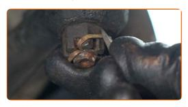
Connect the ABS sensor wiring.
