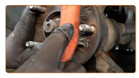
Treat the contacting surface. Use ceramic grease.
