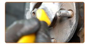
64 Install the brake disc.
