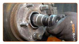
Restake the fastener of the driveshaft. Use a flat metal-working chisel. Use a hammer.
