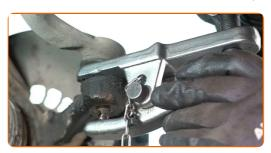
Clean the fasteners connecting the ball joint to the suspension control arm. Use a wire brush. Use WD-40 spray.
