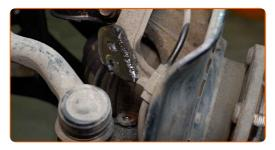
Clean the ABS sensor fastener. Use a wire brush. Use WD-40 spray.
