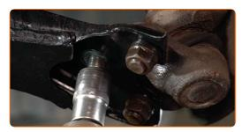
Disconnect the ball joint from the control arm. Use a crowbar.
