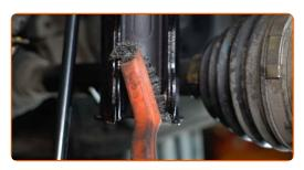
Clean the tie rod end fastener. Use a wire brush. Use WD-40 spray.
