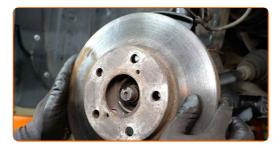
Clean the mounting seat of the brake caliper bracket. Use a wire brush. Use WD-40 spray.
