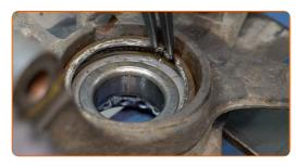
Dismantle the inner bearing race that is remaining on the hub. Use a bush and bearing driver set. Use a bearing separator.
