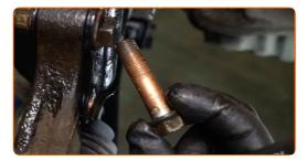
Detach the driveshaft from the steering knuckle.
