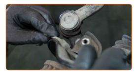
Tighten the fastener of the ABS sensor wiring harness. Use a drive socket #10. Use a torque wrench. Tighten it to 8 Nm torque.
