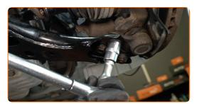
Tighten the brake caliper bracket fasteners. Use a drive socket #17. Use a torque wrench. Tighten it to 106 Nm torque.
