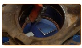
Press the new bearing in the steering knuckle. Use a bush and bearing driver set.
