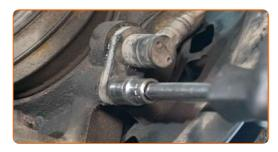
Tighten the fasteners connecting the ball joint to the control arm. Use a drive socket #17. Use a torque wrench. Tighten it to 75 Nm torque.
