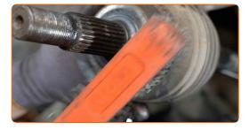
Treat the splines of the driveshaft CV joint. Use copper grease.
