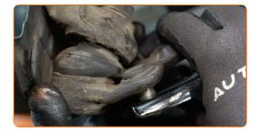
Tighten the fasteners that connect the ball joint to the suspension arm. Use a drive socket #17. Use a ratchet wrench.
