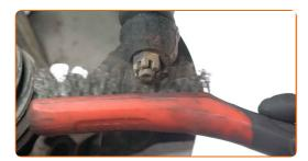
Unscrew the end fastening nut to the steering knuckle. Use a drive socket #17. Use a ratchet wrench.
