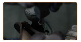
Treat the mounting surface of the ABS sensor. Use a multipurpose grease.
