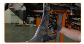
Clean the suspension arm mounting seats. Use a wire brush. Use WD-40 spray.
