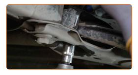
8 Remove the fastening bolt.
