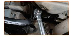
Tighten the rear fastener connecting the arm to the body subframe. Use a combination spanner #19. Use a drive socket #19. Use a torque wrench. Tighten it to 137 Nm torque.
