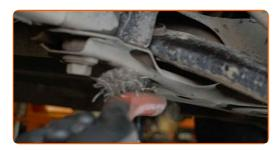
Unscrew the rear fastener connecting the control arm to the subframe. Use a combination spanner #19. Use a drive socket #19. Use a ratchet wrench.
