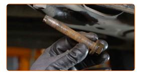
Clean the front fastener that connects the suspension arm to the subframe. Use a wire brush. Use WD-40 spray.
