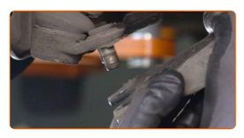
Remove the fastening bolt.
