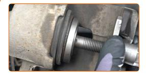
18 Install the brake caliper and fix it.
