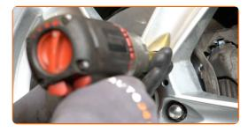
Lower the car and working in a cross order, tighten the wheel bolts. Use wheel impact socket #19. Use a torque wrench. Tighten it to 103 Nm torque.
