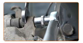
**32** Tighten the brake caliper bracket fasteners. Use a drive socket #17. Use a torque wrench. Tighten it to 106 nm torque.
