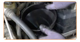
Pour oil into the engine through the filler. Required amount of oil: 4,20 l.
