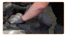
Release the air filter cover clips.
