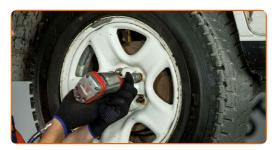
Lower the car and working in a cross order, tighten the wheel bolts. Use wheel impact socket #17. Use a torque wrench. Tighten it to 103 nm torque.
