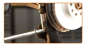
Tighten the fastening nut connecting the tie rod end to the steering knuckle. Use a drive socket #17. Use a torque wrench. Tighten it to 49 nm torque.
