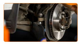
Install the cotter pin fixing the tie rod end fastening. Use nippers.
