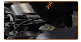
Unscrew the filter housing cap together with the old filter element. Use the 76-14F socket. Use a ratchet wrench.
