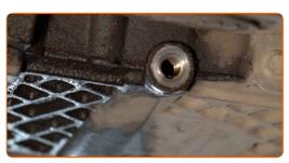
Screw in the new drainage plug and tighten it. Use a drive socket #13. Use a torque wrench. Tighten it to 25 Nm torque.
