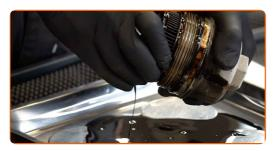
Remove the oil filter cover O-ring.
