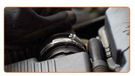
Screw in the fastening screws of the air filter cover. Use a drive socket #8. Use a ratchet wrench.
