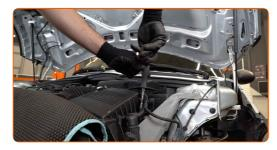
Remove the fender protection cover.
