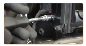
Treat the connector of the power mirror switch. Use dielectric grease.
