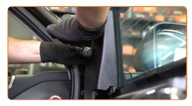
Attach the power window connector to the switch module.
