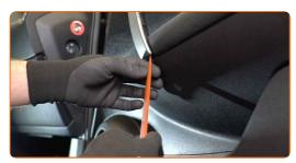
Unscrew the door handle fastener. Use a drive socket #10. Use a ratchet wrench.
