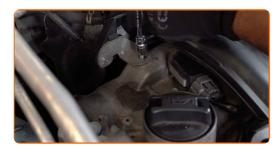
Attach the vacuum booster hose to the intake manifold.
