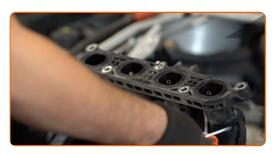
Remove the intake manifold gasket. Use a flat screwdriver.
