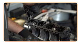
Install the new intake manifold gasket.
