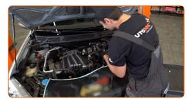
Unscrew the fasteners connecting the throttle valve to the intake manifold. Use a drive socket #8. Use a ratchet wrench.
