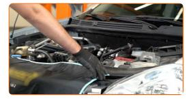
Disconnect the crankcase ventilation hose from the air duct. Use round-nose pliers.
