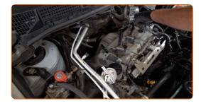
Clean dirt, dust and debris from inside the spark plug well.
