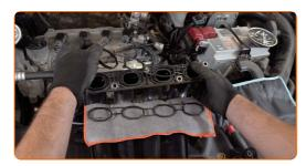
27 Install the intake manifold.
