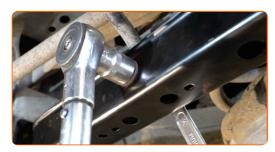
Remove the support from under the arm.
