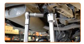
Tighten the top shock absorber fastening. Use a drive socket #16. Use a torque wrench. Tighten it to 70 Nm torque.
