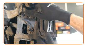
Tighten the brake caliper bracket. Use a drive socket #17. Use a torque wrench. Tighten it to 84 Nm torque.
