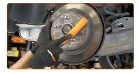
16 Remove the brake disc.
