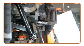
Remove the caliper bracket.
