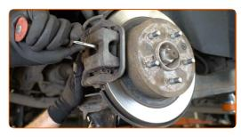
10 Remove the brake caliper.
