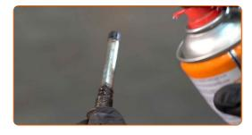
Treat the brake caliper guide pins. Use the brake caliper guide pin grease.
