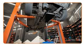
Unscrew the drain plug. Use a drive socket no.19 Or ring spanner no.19.
