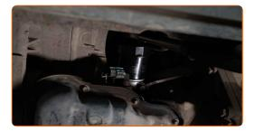
Remove the oil filter. Prepare a container for the old oil filter. Put the old oil filter in the container.
