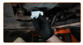
Screw in the new drainage plug and tighten it. Use a torque wrench. Tighten it to 34 nm torque.
