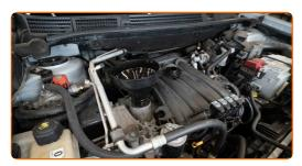
Pour oil into the engine through the filler. Required amount of oil: 4.3 L.
