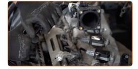
Tighten the intake manifold fasteners. Use a drive socket #10. Use a torque wrench. Tighten it to 27 nm torque.
