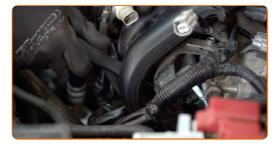
Tighten the fasteners of the intake manifold bracket. Use a drive socket #10. Use a torque wrench. Tighten it to 10 nm torque.
