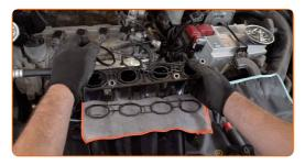
24 Install the intake manifold.
