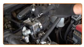
Disconnect the air intake pipe from the air filter housing.
