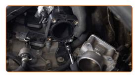
Detach the vacuum booster hose from the intake manifold.
