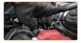
Tighten the clamp and the fasteners on the air filter intake pipe. Use a drive socket #10. Use a ratchet wrench.
