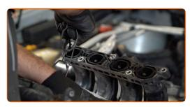
23 Install the new intake manifold gasket.
