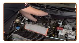
Plug in the ignition coil connector.
