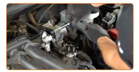
Release the clamp and detach the connector and the vacuum hose from the intake manifold near the throttle valve. Use round-nose pliers.
