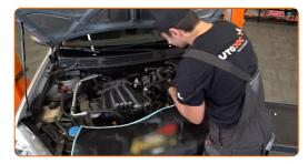
Unscrew the fasteners connecting the throttle valve to the intake manifold. Use a drive socket #8. Use a ratchet wrench.
