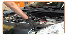
Disconnect the crankcase ventilation hose from the air duct. Use round-nose pliers.
