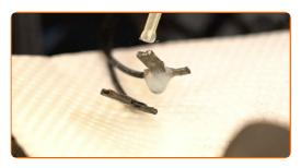
8 Attach the mirror heating connectors.
