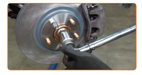
Install the CV axle nut cotter pin. Use a hammer.
