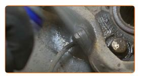
Unscrew the ABS sensor fastener. Use a drive socket #10. Use a ratchet wrench.
