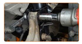
Disconnect the steering knuckle from the shock absorber strut.
