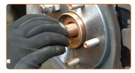
Tighten the drive shaft nut. Use a drive socket #32. Use a torque wrench. Tighten it to 185 nm torque.
