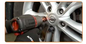
Lower the car and working in a cross order, tighten the wheel bolts. Use wheel impact socket #21. Use a torque wrench. Tighten it to 112 Nm torque.
