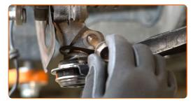
Screw the fasteners of the ball joint. Use a combination spanner #18. Use a drive socket #18. Use a tap wrench.
