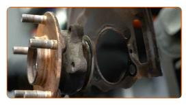
Clean the hub bearing mounting seat. Use a wire brush.
