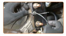
Attach the ABS sensor connector.
