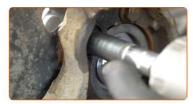
Tighten the hub. Use a drive socket #17. Use a torque wrench. Tighten it to 70 nm torque.
