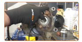
Release the vice and take out the wheel hub together with the bearing.
