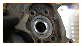
Screw the wheel hub axle nut. Use a drive socket #17. Use a ratchet wrench.
