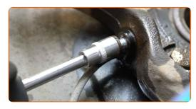
Disconnect the ABS sensor. Use a flat screwdriver. Use water pump pliers.
