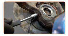
Treat the fasteners of the wheel hub bearing. Use copper grease.
