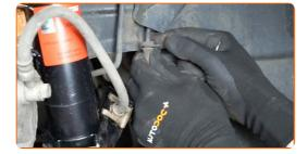
Remove the wheel arch cover. Use a clip removal tool.
