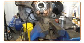
Install the steering knuckle with a hub in assembly.
