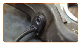
Tighten the fastener that connects the ABS sensor to the steering knuckle. Use a drive socket #10. Use a torque wrench. Tighten it to 13 nm torque.
