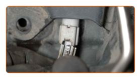
Unscrew the lower fastener connecting the shock strut to the steering knuckle. Use a combination spanner #18. Use a drive socket #21. Use a ratchet wrench.
