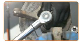
Treat the ABS sensor fastener. Use a multipurpose grease.
