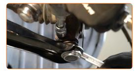
Connect the tie rod end to the steering knuckle.
