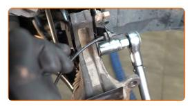
Clean the hub. Treat the contacting surface. Use copper grease.
