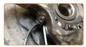
Unscrew the wheel hub axle nut. Use a drive socket #17. Use a ratchet wrench. Use a tap wrench.
