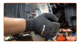
Unscrew the ball joint fastening to the steering knuckle. Use a combination spanner #18. Use a drive socket #18. Use a tap wrench.
