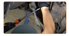
Tighten the fastener connecting the stabilizer link to the shock strut. Use a combination spanner #19. Use a drive socket #19. Use a torque wrench. Tighten it to 65 Nm torque.
