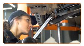
Tighten the front fastener connecting the control arm to the subframe. Use a drive socket #21. Use a torque wrench. Tighten it to 171 Nm torque.
