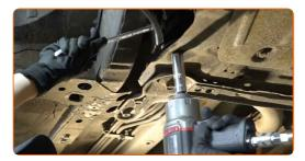
Tighten the rear fastener connecting the arm to the body subframe. Use a combination spanner #18. Use a drive socket #18. Use a torque wrench. Tighten it to 98 Nm torque.
