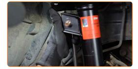
Tighten the fastener connecting the stabilizer link to the shock strut. Use a drive socket #19. Use a torque wrench. Tighten it to 65 Nm torque.
