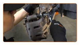
10 Remove the brake caliper.
