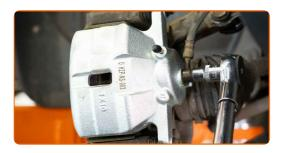
Remove the brake hose clamp.
