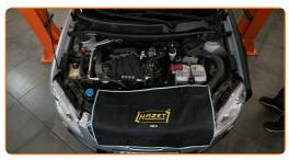
Unscrew the brake fluid reservoir cap.
