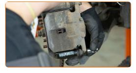
16 Remove the brake caliper.
