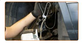
Fasten the brake hose on the strut. Install the brake hose retaining clip. Use a hammer.
