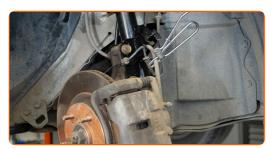
Unscrew the brake hose from the brake caliper. Use a drive socket #12. Use a ratchet wrench.
