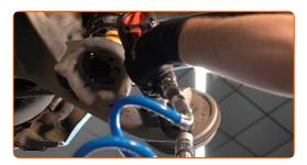
Tighten the lower fastener of the shock absorber. Use a drive socket #18. Use a torque wrench. Tighten it to 90 Nm torque.
