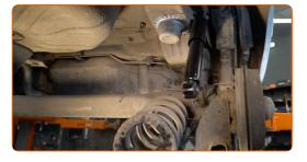
Remove the rubber spring spacer.
