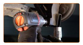
9 Remove the fastening bolt.
