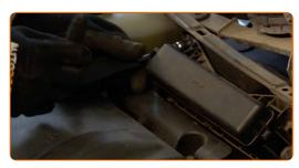
Remove the panel assembled with the windscreen wiper linkage.
