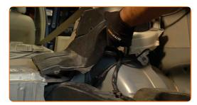
Loosen the upper fastener of the shock strut mount. Use a drive socket #14. Use a ratchet wrench.
