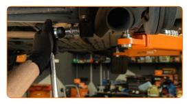
Unscrew the top fastening of the shock strut mount. Use a drive socket #14. Use a ratchet wrench.
