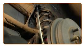
Remove the suspension strut. Use a crowbar.
