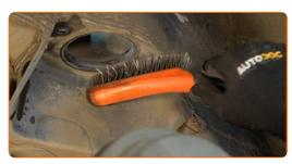
Treat the mounting seats of the shock strut. Use copper grease.
