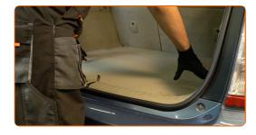
Install the clips of the boot front lower lining.
