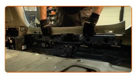
Unscrew the fastener and remove the boot side sound insulation. Use a drive socket #10. Use a ratchet wrench.
