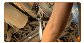
Tighten the lower fastening of the shock absorber. Use a drive socket #19. Use a torque wrench. Tighten it to 80 Nm torque.
