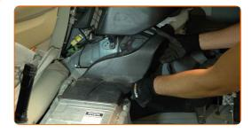
Install the boot side sound insulation and screw in its fasteners. Use a drive socket #10. Use a ratchet wrench.
