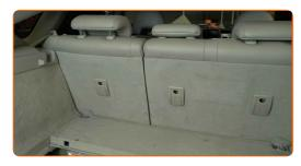
65 Install the boot front lower lining.
