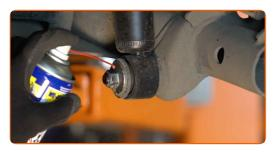
Unscrew the lower fastener of the shock absorber strut. Use a drive socket #19. Use a ratchet wrench.
