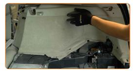
Screw in the fastener of the boot side lining. Use a drive socket #10. Use a ratchet wrench.
