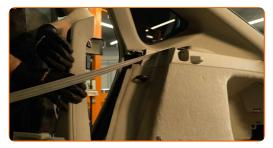
Unscrew the fasteners of the side plastic trim panel. Use a drive socket #10. Use a ratchet wrench.
