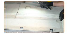
Screw in the fastener of the central protective plastic panel. Use a drive socket #10. Use a ratchet wrench.
