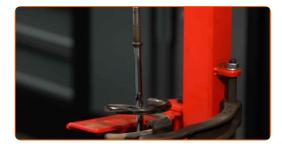
Release the coil spring.
