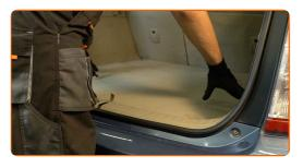
Install the clips of the boot front lower lining.
