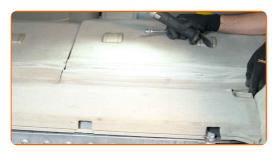
Screw in the fastener of the central protective plastic panel. Use a drive socket #10. Use a ratchet wrench.
