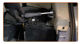
Screw in the fastener of the boot side lining. Use a drive socket #10. Use a ratchet wrench.
