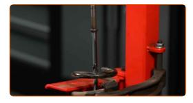
Release the coil spring.
