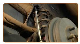
Remove the suspension strut. Use a crowbar.
