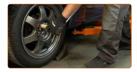
Tighten the upper fastener of the shock absorber strut mount. Use a drive socket #14. Use a torque wrench. Tighten it to 55 Nm torque.
