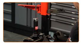
Install the spring on the shock absorber.
