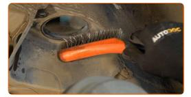
Treat the mounting seats of the shock strut. Use copper grease.
