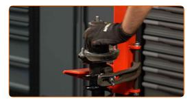
Tighten the shock strut piston rod nut. Use a drive socket #17. Use HEX No.H6. Use a torque wrench. Tighten it to 56 Nm torque.
