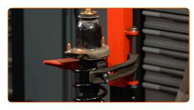
Remove the assembled shock strut.
