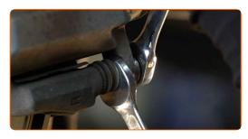
10 Remove the brake caliper.
