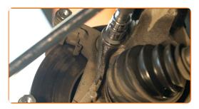
Remove the caliper bracket.
