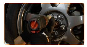
Lower the car and working in a cross order, tighten the wheel bolts. Use a torque wrench. Tighten it to 103 Nm torque.
