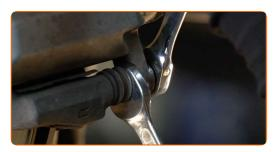
10 Remove the brake caliper.
