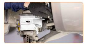
Tighten the fastener connecting the brake pipe to the brake caliper. Use a drive socket #14. Use a torque wrench. Tighten it to 33 Nm torque.
