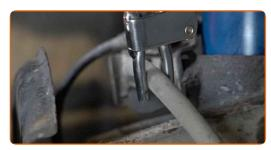
Unscrew the brake hose from the brake caliper. Use a drive socket #14. Use a ratchet wrench.
