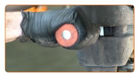
Remove the brake caliper.
