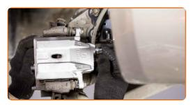
Clean dirt from the brake hose bolt. Use a brake cleaner.
