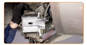
Tighten the brake caliper bleed screw. Use a combination spanner #9. Use a torque wrench. Tighten it to 8 Nm torque.
