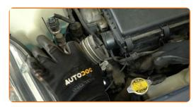
6.1 Loosen the tensioner lever of the V-ribbed belt.
