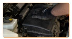
Press the air filter cover clips into place.
