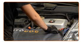
Release the air filter cover clips.
