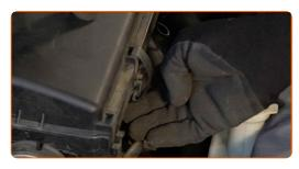
Remove the fender protection cover.
