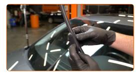
6 Remove the blade from the wiper arm.
