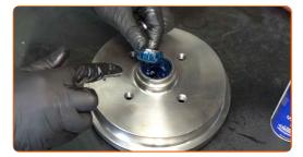
Install the brake drum assembled with the wheel hub bearing.
