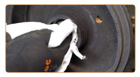
Remove the inner race of the wheel bearing from the brake drum. Use a flat metal-working chisel. Use a hammer.
