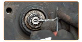
Unscrew the hub nut. Use a drive socket #30. Use a ratchet wrench.
