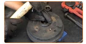
Clean the hub bearing mounting seat. Use WD-40 spray.
