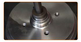
Treat the inner race and the wheel bearing. Use a multipurpose grease.
