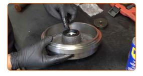
25 Install a new hub bearing and secure it.
