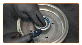
Install the wheel hub bearing retaining ring. Use a bush and bearing driver set. Use a hammer.
