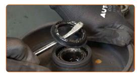
Remove the hub bearing mounting. Use a crowbar.
