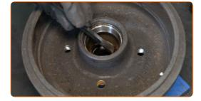
Remove the inner race of the wheel bearing from the brake drum. Use a flat metal-working chisel. Use a hammer.
