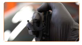
Remove the blade from the wiper arm.
